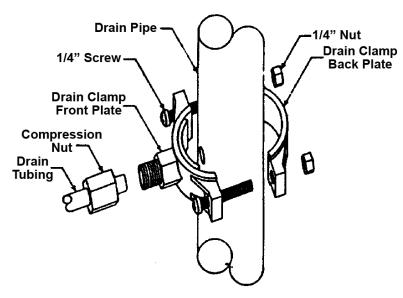
NOTE: Some states require the use of an air gap faucet. Check your local plumbing code to assure compliance. Locate the drain connection away from the garbage disposal to prevent potential contamination and system fouling.
