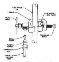
Do not over tighten the clamp. The clamp should be secure and resist a slight twisting force. Turn the saddle-tapping valve clockwise until the needle fully pierces the tubing and the valve seats. For maximum flow, back the handle out all the way. Adjust as required.
